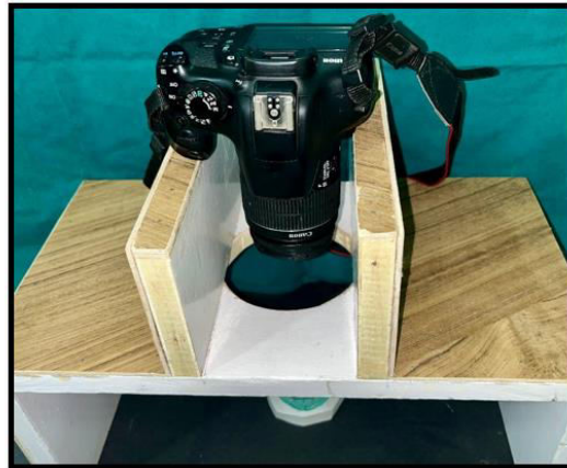
Fig. 6 – Set up for Cast Photography
